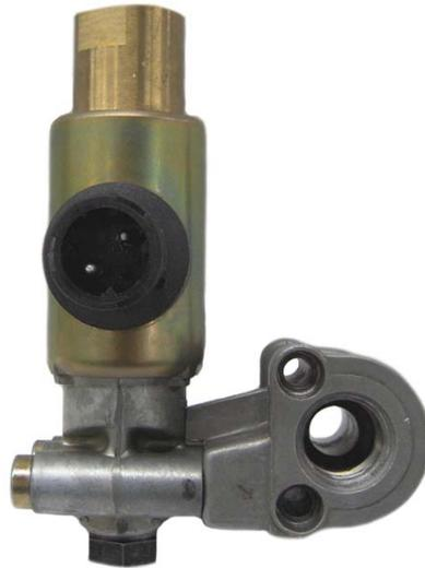
*When the ATC Valve is installed with the whole ABS valve package, the ATC Valve is attached to the Relay Valve*
